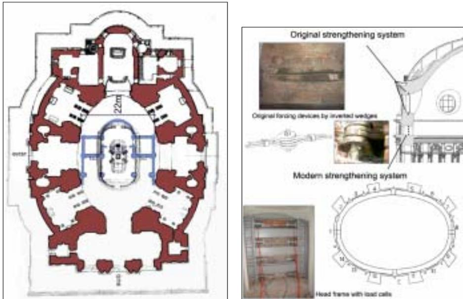
Figure 3. (a) Plan of the Sanctuary and ancient church, (b) Annular iron strengthening applied by Gallo (1732) and modern strengthening system (1987)
