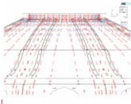
Figure 6. Vectorial representation of principal stresses: detail of the dome.
