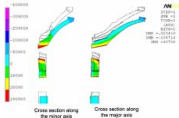
Figure 7. Diagram of the stresses normal to the sections along the minor and the major axis of the dome.
