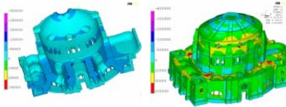
Figure 5. (a) Diagram of principal (sub-vertical) stresses S3. (b) Diagram of principal (sub-horizontal) stresses S1
