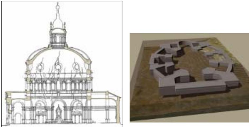
Figure 2. (a)Cracks in the dome. North-south section; view of the west side (Garro 1962). (b) Axonometric view of foundation and foundation layers
